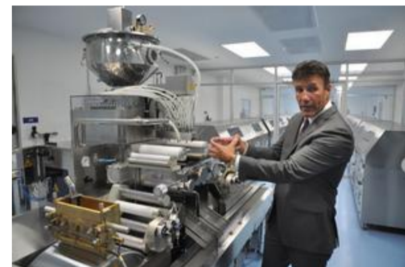
Nutri-Force President and CEO Anthony Alfonso explains how a machine forms and fills softgel capsules.
